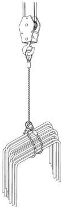
**Fig.13 Choker hitch double wrapped**
