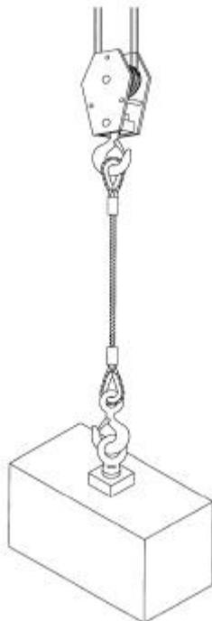
**Fig. 9 Vertical or straight lift**
